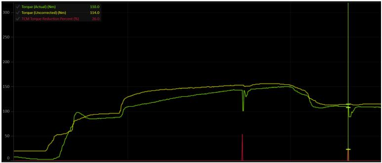
Note the channel name for the reduction request has since changed to "TCM Torque Reduction Request".
